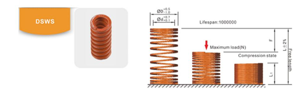
Maximum Iload calculate method: Maximum Iload=compression×spring constant N=Fmm×N/mm (kgf=N×0.101972) Maximum Iload Deviation:+20% to -10%
